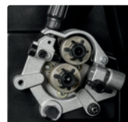
Heavy-duty aluminum two-drive-roll system
