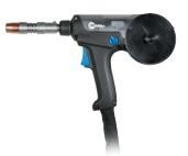
Spoolmate<sup>™</sup> 200 Spool Gun 300497 Reliable and economical spool gun perfect for hobbyists and light fabricators who weld aluminum. Handles .030–.035 inch (0.8–0.9 mm) aluminum wires and .023–.035 inch (0.6–0.9 mm) steel/stainless steel wires. Rated at 160 amps, 60 percent duty cycle with 20-foot cable assembly. For detailed information, see Spoolmate literature M/1.47. Optional Spoolmate™ 200 Head Tubes30059145-degree head tube3005929-inch extension head tube2433855-inch head tube
