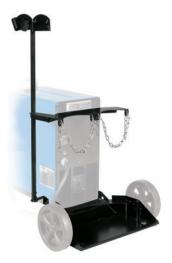
Dual EZ-Change<sup>™</sup> Low Cylinder Rack with Elevated Gun and Cable Rack 300337 Dual cylinder rack allows operators to easily roll cylinders on and off the rack with no lifting. Gun and cable rack keeps cables off the floor and tangle free.
